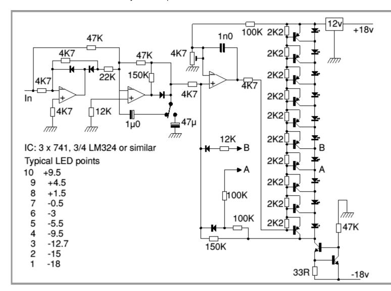
The circuit was designed to work with an audio power amplifier which operated off +18v-0v-18v power rails. The actual voltage used is not too critical except that the feedback is referred to the LED chain which itself is anchored to a +12v rail, hence the separate stabilizer for this. It has one large advantage over most of the LED chips available - all the LEDs are in series so it only draws 20mA irrespective of the number of LEDs illuminated.
